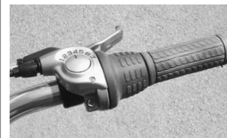
LEFT: A twist-grip changer for the seven-speed hub gear
