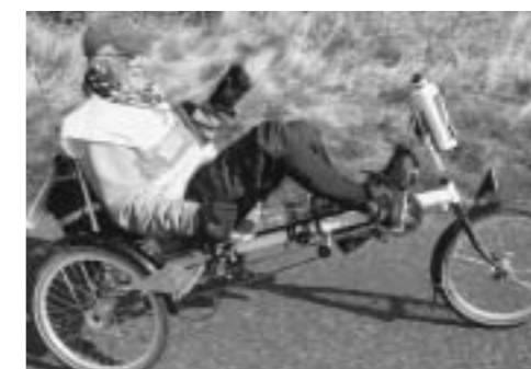
ABOVE: The Hase Kettwiesel is well-suited to special needs use, and a hand-cranked version is available along with many adaptations. Several can be linked together for 'tandem' use too if required.
