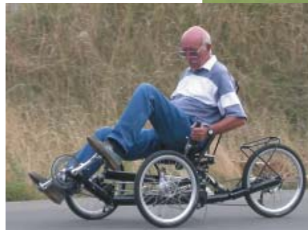
The Trilite folding recumbent trike. A remarkably neat folded package for a three-wheeler.
