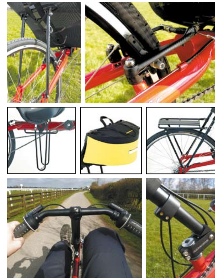
TOP LEFT: Seat angle adjustment is via two telescoping tubes: the rings on the pins look like they should rattle but don't!
