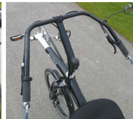
Aluminium side plates (above left) provide mounting points for chain pulley, rack and suspension. The solidly-built rack (above) comes with a basic battery rear light, but the curved sides could be awkward with some panniers. The MEKS carbon fork (far left) adds to steering stability while the wide 'aero' bars (left) offer fingertip control. The bar end shifters are pleasant to use but easily knocked.
