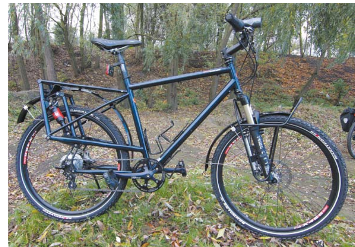
ABOVE CENTRE: The massive rear rack, with braze-ons for a rear light and holes (here sealed with aluminium plugs) for internal dynamo lighting cables.
