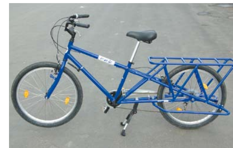
RIGHT: The Yuba offers a large load bed above the wheel, and also rails rated 50 kg each side. These detach easily if required via two bolts ( ABOVE RIGHT ) and a steel clamp block ( ABOVE FAR RIGHT ) each side.
