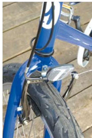
ABOVE: Basic but effective V-brakes do the stopping.
