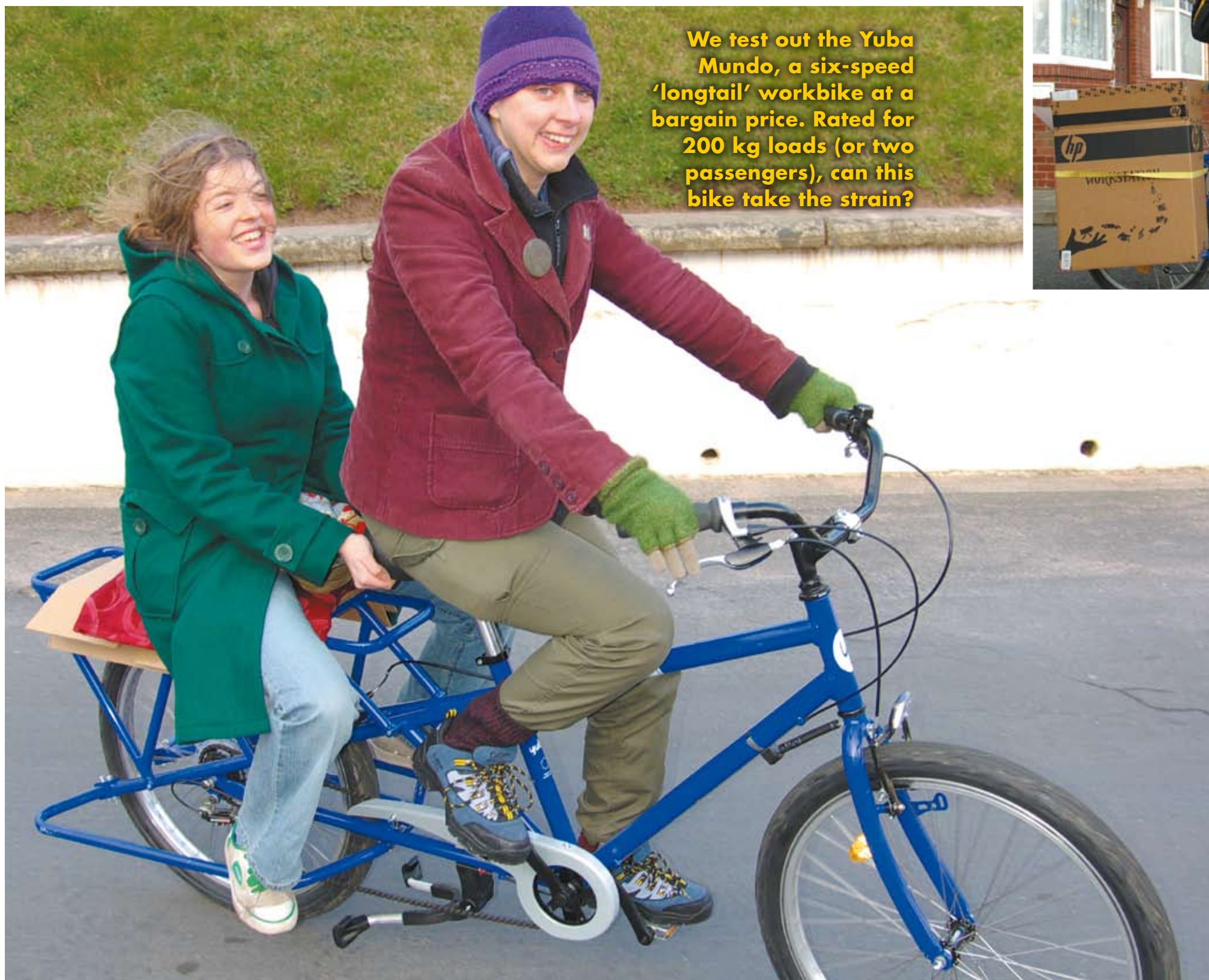
RIGHT: The Yuba offers a large load bed above the wheel, and also rails rated 50 kg each side. These detach easily if required via two bolts ( ABOVE RIGHT ) and a steel clamp block ( ABOVE FAR RIGHT ) each side.
