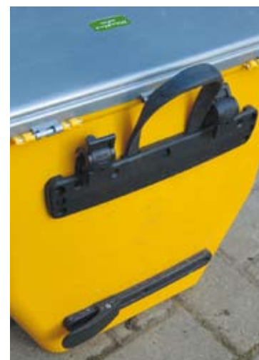
BELOW: The attachment system is bolted securely to the plastic shell, and fits rack rails up to 12 mm.
