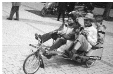
Lissy (right) The Lissy, a two-wheel sociable trike developed by Peter Lis, was almost constantly in action outside the show giving people lifts. The version he had here this year was electric-assisted.
