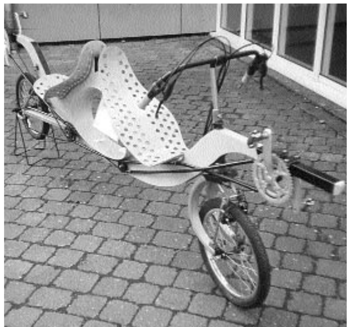
Lissy (right) The Lissy, a two-wheel sociable trike developed by Peter Lis, was almost constantly in action outside the show giving people lifts. The version he had here this year was electric-assisted.
